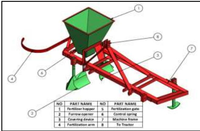
Fig. (2.2): 3D drawing of the tree fertilizing machine.
