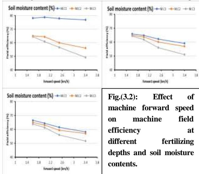
**Fig.(3.2): Effect of machine forward speed on machine field efficiency at different fertilizing depths and soil moisture contents.**
