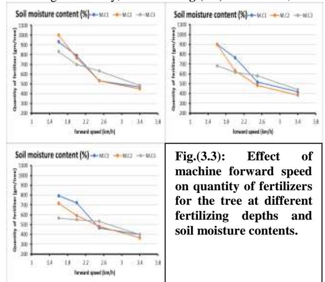
**Fig.(3.3): Effect of machine forward speed on quantity of fertilizers for the tree at different fertilizing depths and soil moisture contents.**
