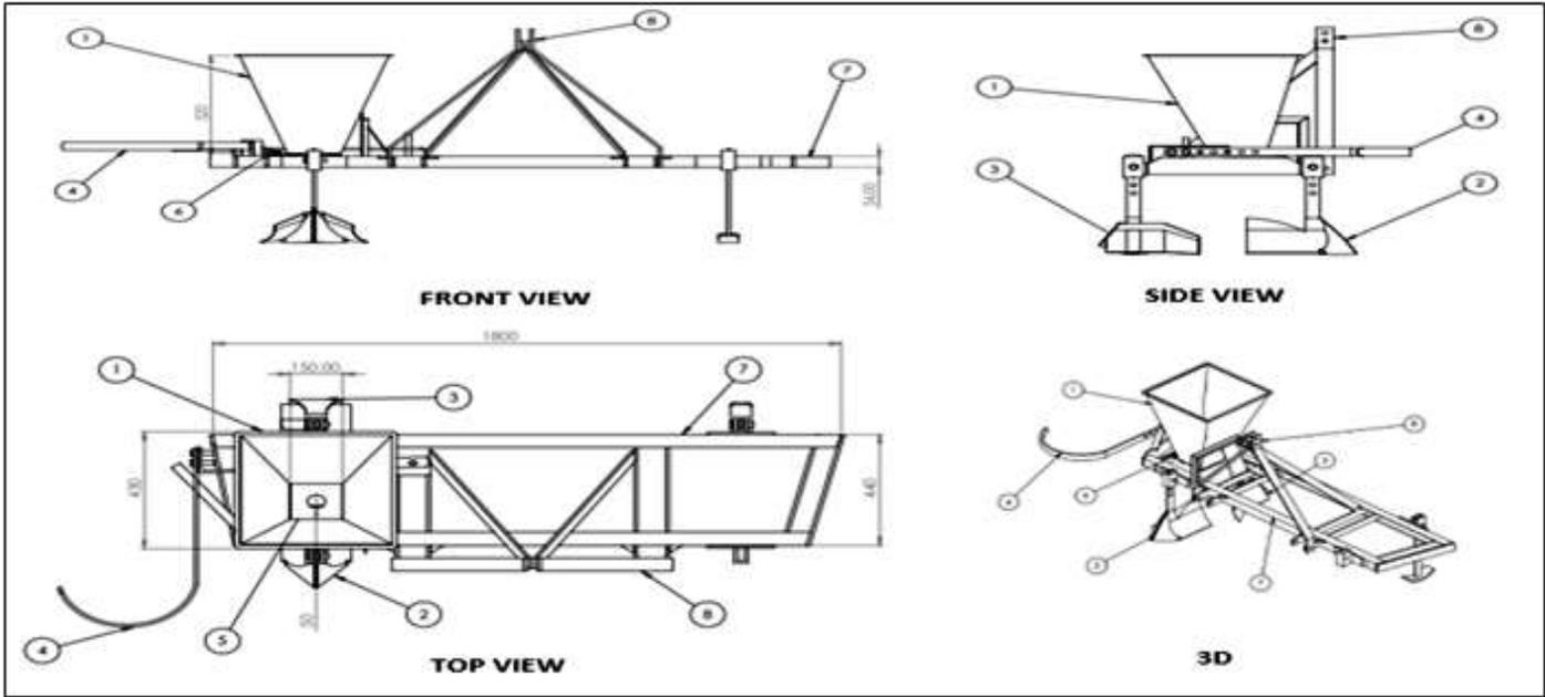
Fig. (2.3): Engineering drawing of the tree fertilizing machine
